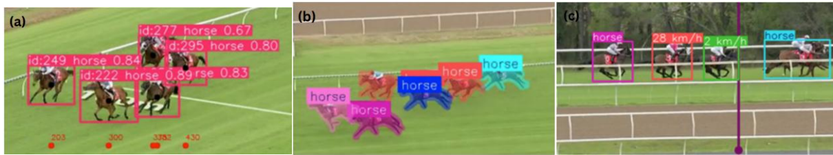
Figure 2: YOLOv11 (a) with centroids (b) Instance Segmentation & (c) speed estimation
